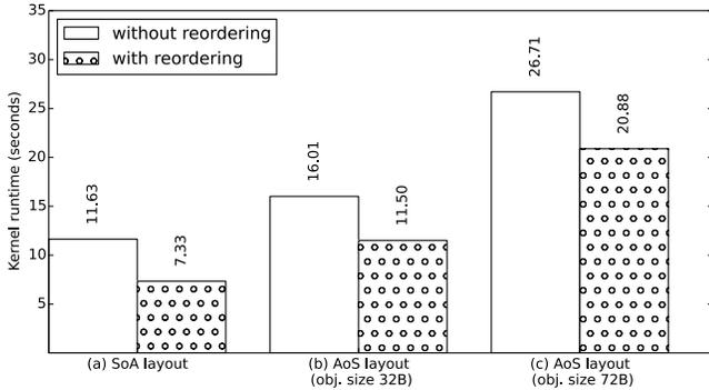
**Figure 8:** Kernel Running Time for Traffic Simulation (CUDA)
