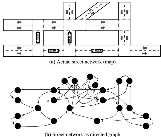
Figure 1: Example: Street Network for Traffic Simulation
