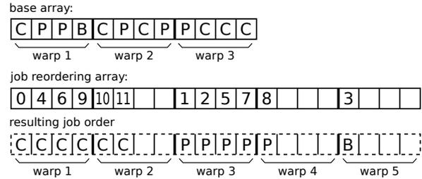
Figure 5: Example: Job Reordering (assuming warp size 4).
