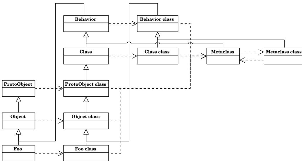
**Figure 4.1.:** Squeak class model. Every class is an instance of its meta class. Meta classes are instances of `Metaclass`. Meta classes and non-meta classes form a helix [22], connecting the meta class hierarchy with the non-meta class hierarchy.
