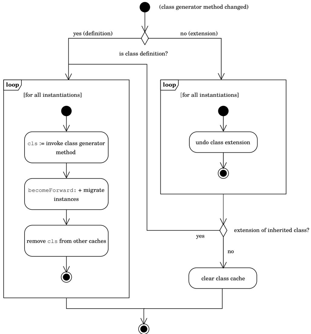
**Figure 4.13.:** High-level overview of the class migration process. Classes and instances are only migrated if the nested class is a class definition or a class extension of an inherited nested class.
