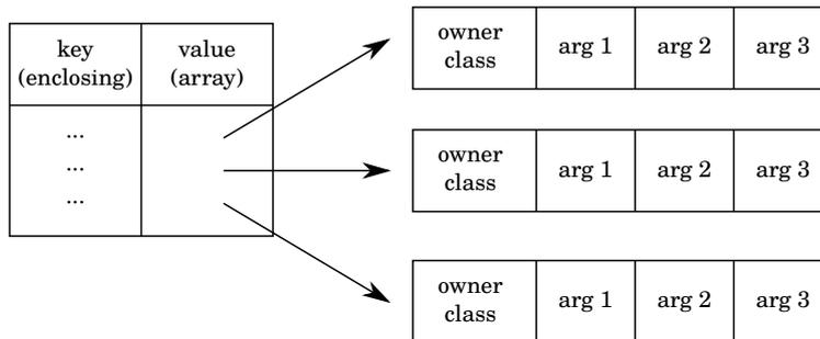
**Figure 4.11.:** Example: Argument cache. The cache is a dictionary mapping parameterized instantiations to an array of arguments that was used to generate the respective class.
