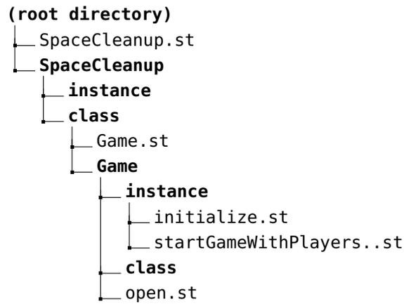
**Figure 4.16.:** Example: Source code export. A module and nested classes are represented by a source code file (class generator method) and a directory containing members. Methods are represented by source code files.
