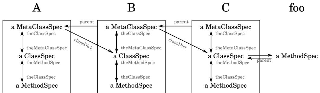
**Figure A.2.:** Example: Detailed meta model. Class B is nested within class A and class C is nested within class B. foo is an instance method of class C. All three entities within a box have the same meta class specification as a parent.
