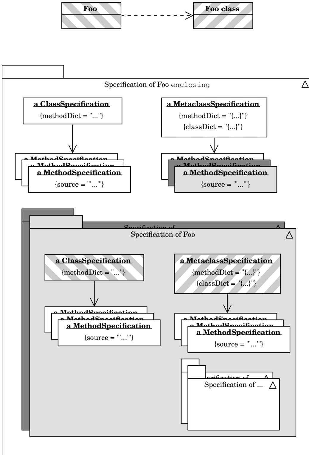
**Figure 4.3.:** Example: Meta model. There is a class specification for Foo and a meta class specification for Foo class (same pattern). Foo’s enclosing class has a method specification (light gray color) defining the class to which the methods are added (target class), in addition to the corresponding class specification.
