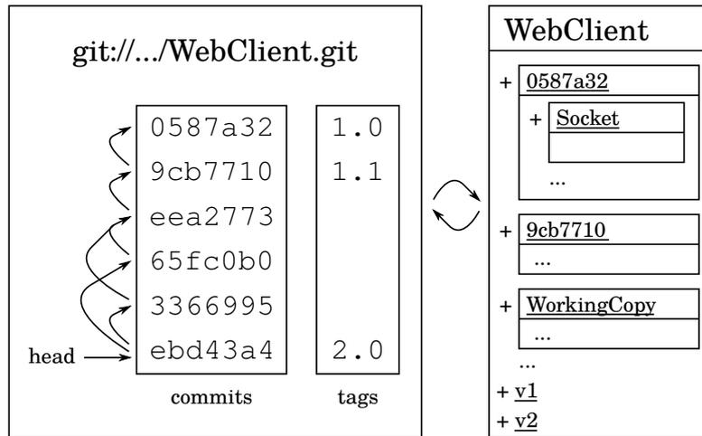
**Figure 7.1:** Example: git-based version control with nested classes. `WebClient` is a module and every commit in the underlying version control system corresponds to an automatically-generated nested class in Matriona.
