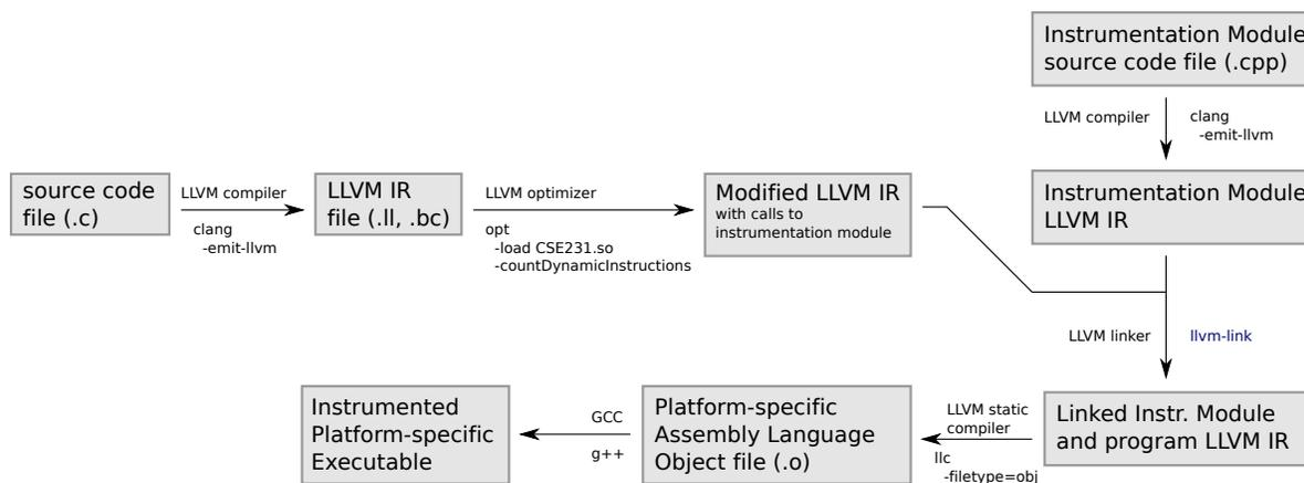
Figure 2: Compilation and linkage workflow for Section 2 and Section 3.
